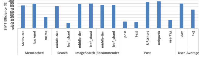
Figure 4: SIMT control efficiency of naive batching for some microservices.
